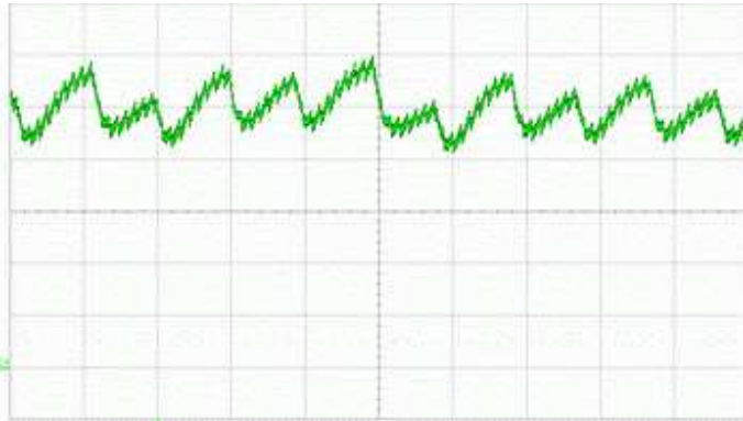
Running current @ 24 V ( I = 500\text{mA/div} ; t = 500\mu\text{s/div} )
