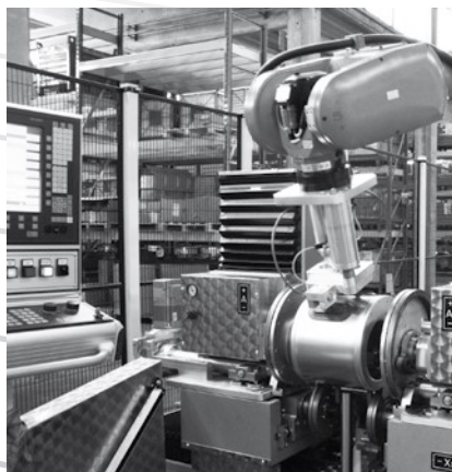
Automated manufacture of compact scroll and impeller with forward curved blades
